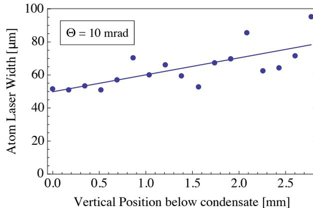
**Figure 4.** The transverse size of the atom laser of the ‘pure’ atom laser of Fig. 1a. The solid line is a straight line fit resulting in a divergence of 10 mrad and an initial size of 50  $\mu\text{m}$ . For comparison: A condensate containing all  $3.1 \times 10^4$  atoms detected in the atom-laser beam would have an axial Thomas–Fermi size of 44  $\mu\text{m}$  in the absence of the dressing rf.
