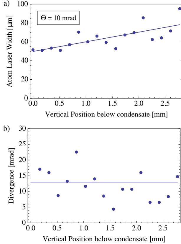
**Figure 8.** Laser width and divergence of the ‘pure’ atom laser of Fig. 1a in real and momentum space. a) the transverse size of the atom laser with the solid line being a straight line fit (for convenience repeated from Fig. 4). b) the divergence of the atom laser based on the velocities assuming as an initial size the Thomas–Fermi radius of 37000 atoms in a trap of  $16.5 \times 561$  Hz trapping frequency ( $44 \mu\text{m}$ ). The solid line is the mean divergence (13 mrad).
