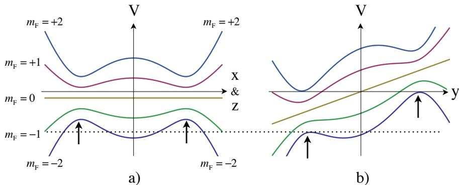
**Figure 2.** The dressed trapping potentials in the presence of gravity. a) depicts the potential in the horizontal directions (not to scale). b) shows the potentials in the direction of gravity. The dotted line denotes the energy, above which gravity pulls the atoms out of the trap. The arrows indicate the positions, where the radio frequency is resonant with local static B-field, i.e. where  $\omega_{\text{rf}} = \Omega_{\text{L}}$ .
