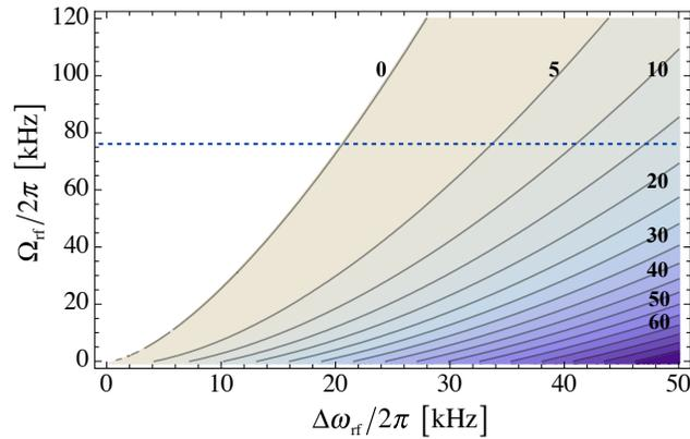
**Figure 7.** The trap depth  $\Delta V_{\text{trap}}$  as a function of  $\Delta\omega_{\text{rf}}$  and  $\Omega_{\text{rf}}$ . In the white region there is no stable trap. The numbers inside the plot denote the values of the corresponding contour line of  $\Delta V_{\text{trap}}$  in kHz. The horizontal dashed line correspond to  $\Omega_{\text{rf}}/2\pi = 76$  kHz, which is the value used in the experiments presented here.
