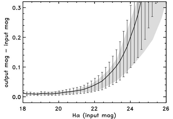
FIG. 1.— Mean of the error distribution of the  $H\alpha$  magnitudes (solid line), and associated  $1\sigma$  uncertainties (error bars), obtained from the comparison between input and output magnitudes in the artificial star experiments. The shaded area shows the distribution of the photometric uncertainties calculated by ALLFRAME.
