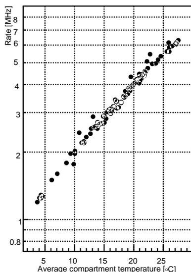
**Figure 5:** An estimate of the dark-count rate obtained from the integration of the normalized sum-spectra versus average compartment temperature, extraction efficiency and dead-time are neglected. The correlation fits very well with the data-sheet.
