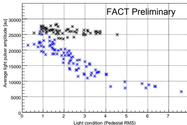
**Figure 1:** The median of the average extracted light-pulser signal versus the measured pedestal rms. The blue asterisk correspond to data taken with only the temperature feedback switched on, the black dots have been taken with the full current feedback enabled.
