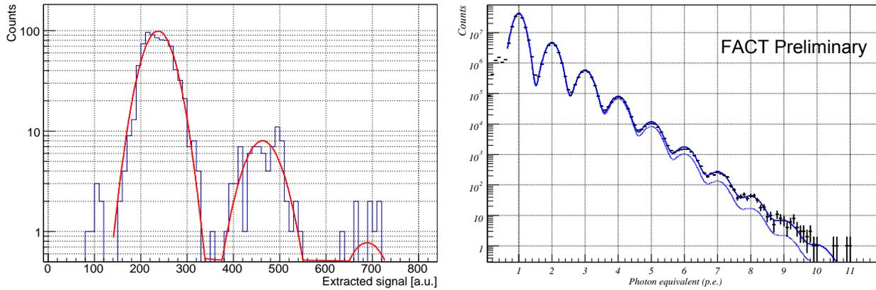
**Figure 3:** Dark count spectrum, for a randomly selected single pixel and a single run (left), and normalized spectrum compiled from all dark count runs and all channels (right). The solid like is a fit with the function explained in the text. For comparison, the dashed line shows a fit with the coefficient  $r$  fixed to zero.
