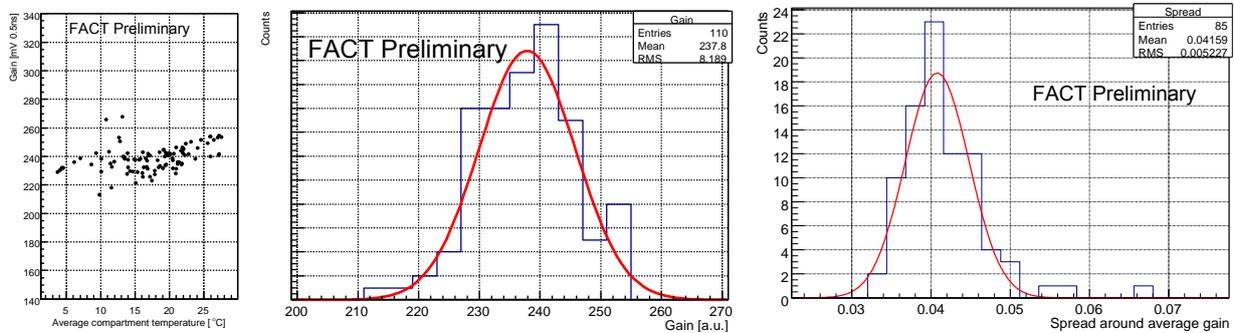
**Figure 4:** Extracted gain (left) versus average compartment temperature (left) and the corresponding projection (middle) with a fitted Gaussian. The right plot shows the corresponding average difference between the gain extracted from the individual channels and the gain obtained from the sum spectrum fitted with a Gaussian.
