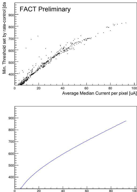
**Figure 3:** Top: Threshold to archive a trigger rate below 70 Hz as determined by a mini-ratescan versus median current, applied for several month before each 5 min data run. Bottom: Trigger threshold depending on median current determined from the parametrized ratescans shown at the top in Fig. 2 (bottom) for a fixed rate of 70 Hz. A good agreement with the measurement in the top figure is visible.
