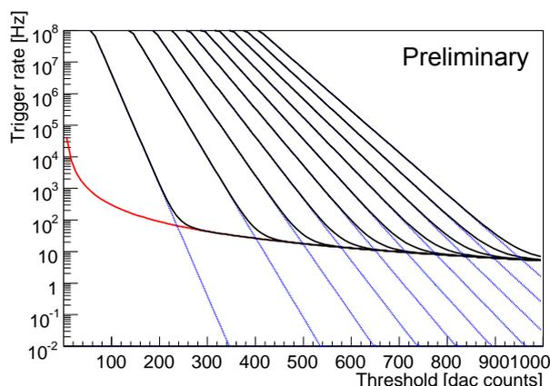
**Figure 2:** Top: Ratescans taken close to zenith at different light conditions between dark night conditions and almost full moon conditions. Bottom: Parametrization for ratescans depending on the measured median current with  $10\mu\text{A}/\text{ch}$  spacing. The power-law of the proton spectrum (red) and the background spectra (black).
