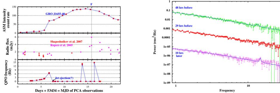
**Figure 4.** The variation of X-ray intensity, Radio flux and QPO frequencies observed for the BH source GRO J1655–40 (2005 outburst) is shown on the left side, while the evolution of power spectra during the peak flare is shown on the right side.
