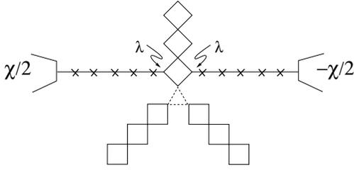
Fig. 3: Sketch of the circuit probing  $m(D)$ : the rhombus at the endpoints of one chain is symmetrically coupled to two one-dimensional Josephson junction arrays connected to two bulk superconductors, whose phase difference is  $\chi$ . At fixed  $\chi$ , the dc Josephson current across the one-dimensional Josephson arrays is  $\propto m(D)$ .
