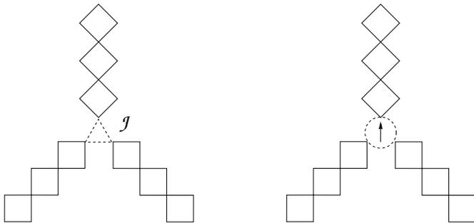
Fig. 2: **a)**  $Y$  junction of three rhombi chains: the spins at the endpoints of the three chains are coupled to each other, with an effective coupling strength  $\mathcal{J}$ ; **b)** representation of the central region by an effective spin-1/2
