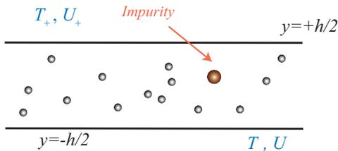
FIG. 1. We observe here a sketch of the system. In this case the impurity is represented as a particle bigger than the gas particles. Energy is input in the system from the boundaries, which consist of two infinite parallel walls with temperature and shear sources.
