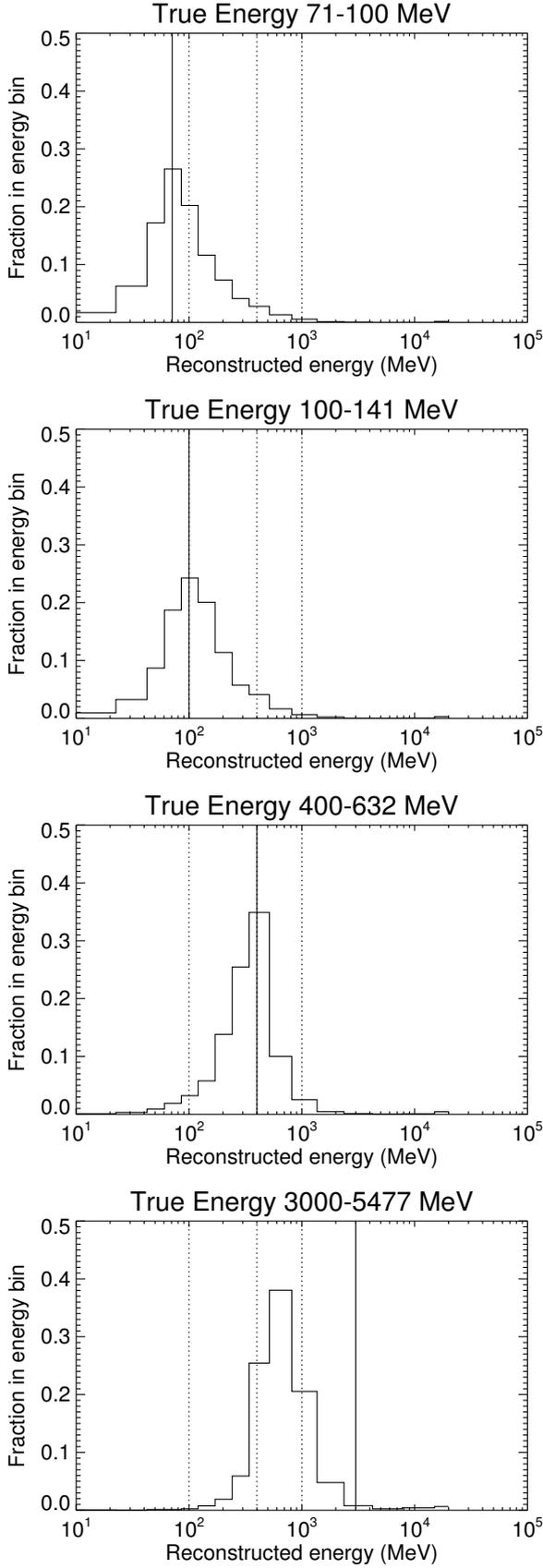
**Fig. 3.** EDPs for filter FMG at various energy bins (71-100, 100-141, 400-632, and 3000-5477 MeV) at  $\Theta = 30^\circ$ . Within each bin the true energy follows a power-law distribution (see Sect. 3.2). The solid vertical line is the lower boundary of the true energy bin, while the dotted lines are fixed at 100, 400, and 1000 MeV.
