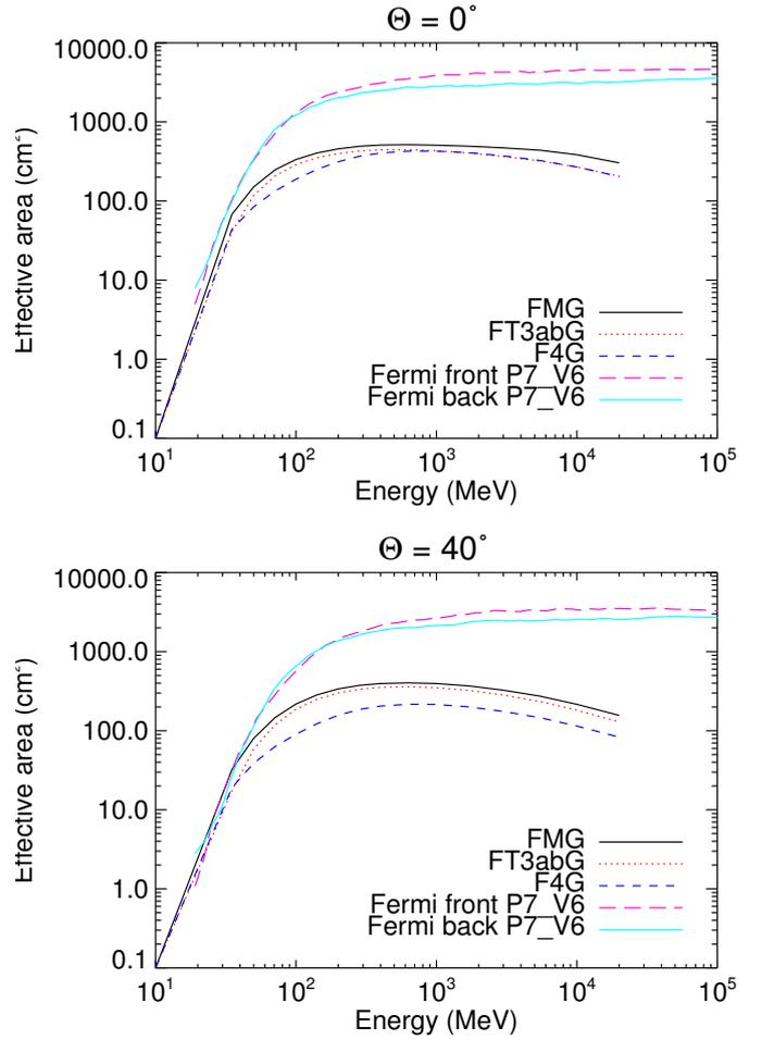
**Fig. 2.** AGILE and Fermi effective areas as a function of energy. The top plot is for  $\Theta = 0^\circ$ , the bottom plot for  $\Theta = 40^\circ$ . AGILE curves are for filters FT3ab and FM3.119, event class G. Fermi Pass 7 curves are for version 6, SOURCE event class, front and back events. Fermi IRFs are taken from the Fermi Science Tools, version v9r23p1. The current version is available for public download at <http://fermi.gsfc.nasa.gov/ssc/data/analysis/software/>.
