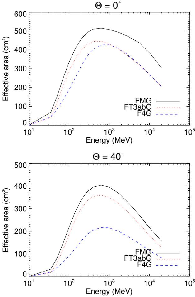
**Fig. 1.** AGILE effective areas as a function of energy. Effective area = geometric area  $\times$  fraction of surviving events. The top plot is for  $\Theta = 0^\circ$ , the bottom plot for  $\Theta = 40^\circ$ . AGILE curves are for filters FT3ab and FM3.119, event class G.
