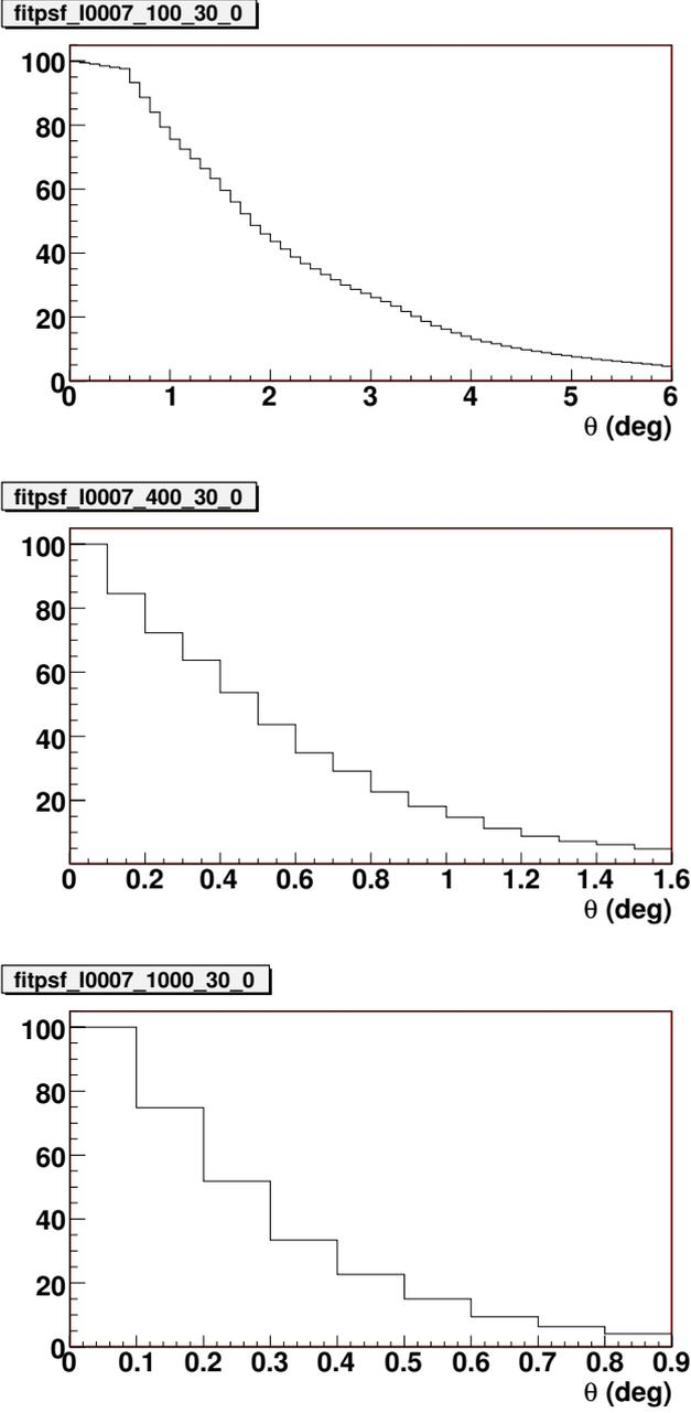
**Fig. 5.** Monoenergetic PSFs at  $\Theta = 30^\circ$  with filter FMG at 100, 400, and 1000 MeV. The I0007 PSF matrices were created by directly binning the Monte Carlo data, dividing the raw histogram by  $\sin \theta$ , and normalizing. The I0010 PSF matrices are identical to those of I0007.
