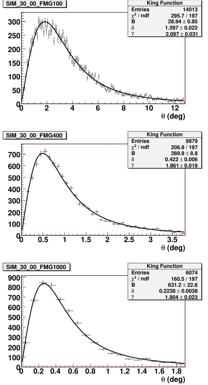
**Fig. 6.** Monoenergetic PSFs at  $\Theta = 30^\circ$  with filter FMG at 100, 400, and 1000 MeV. The I0023 PSF matrices were created by first fitting Eq. (11) to the Monte Carlo data, then binning the values of the King function and normalizing.
