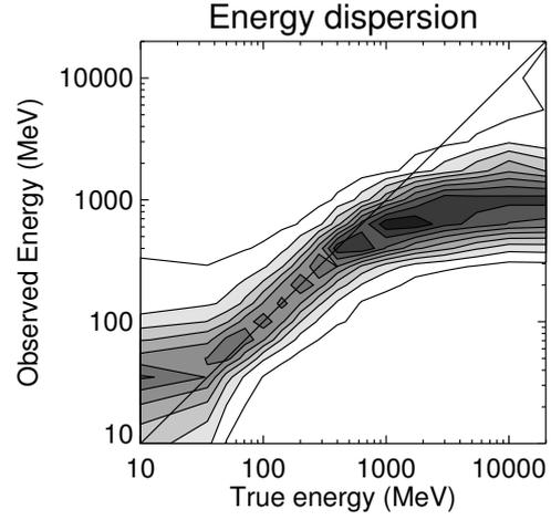
**Fig. 4.** EDP for filter FMG at  $\Theta = 30^\circ$ . Note the deviations from linearity below 100 MeV and above 400 MeV.
