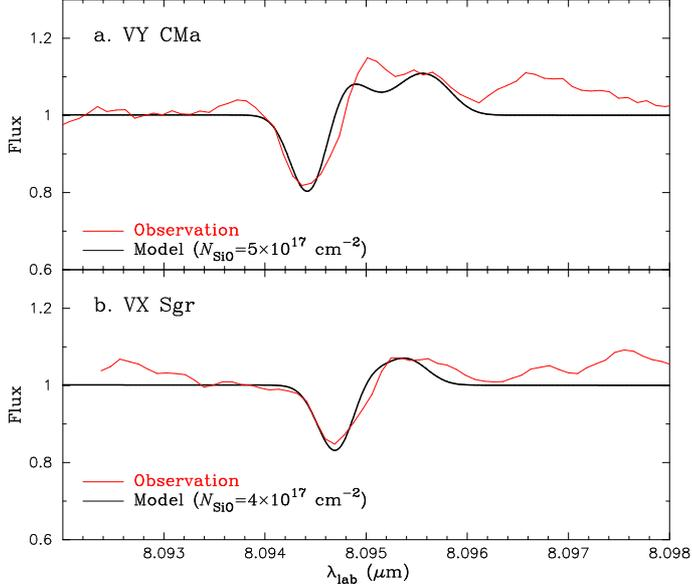
**Fig. 4.** Modeling of the P-Cyg profile of the SiO line 1 – 0  $R(3)$  observed in VY CMa (panel a) and VX Sgr (panel b). In each panel, the red solid line represents the observed spectrum, while the black solid line represents the model spectrum.
