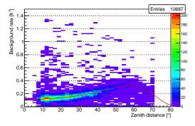
**Figure 1**: Background rate after cuts versus zenith distance. The colour code represents the number of runs, where one run comprises five minutes. For the study, almost 900 hours of data have been used. Details on how this background rate is determined can be found in section 4.
