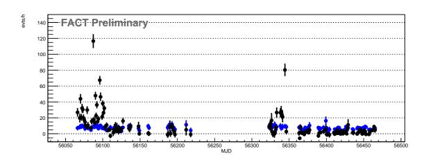
**Figure 2**: Rates for Mrk 501 from May 2012 until June 2013 with one bin per night. In black: Rate of excess events. In blue: Rate of background events. The curves are not yet corrected for the effects of the zenith distance and of ambient light like the moon. The gap in the middle of the curve is due to the source being below the horizon or only visible at very big zenith distance. In June 2012 a big outburst can be seen, see in detail figure 4, and another one in February 2013.
