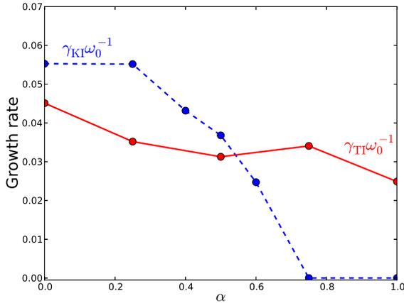
FIG. 5.— Linear growth rates of the fastest growing modes for the tearing (for  $\gamma_{\text{TI}}(k_x = 0.58)$ , red solid line) and the kink (for  $\gamma_{\text{KI}}(k_z = 0.67)$ , blue dashed line) instabilities multiplied by  $\omega_0^{-1}$ , as a function of the guide field strength  $\alpha$ . Each dot represents one simulation. The analysis of the kink/tearing instability was performed using the set of 2D simulations in the  $yz$ - $xy$ -plane.
