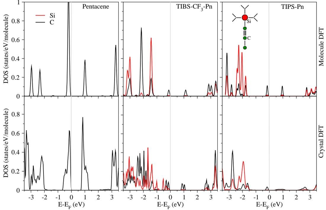
FIG. 2: Comparison of the pentacene DOS with TIBS-CF<sub>3</sub>-Pn and TIPS-Pn in both molecular and crystalline forms.
