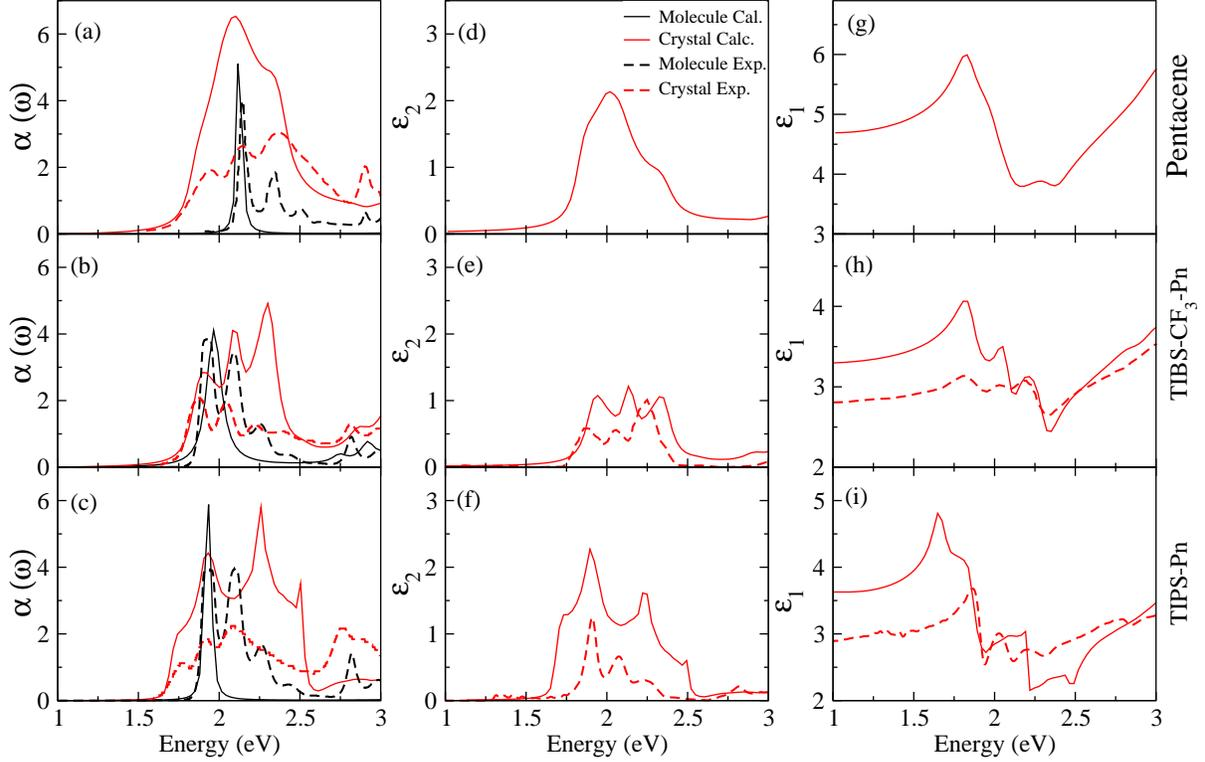
FIG. 3: Spectra of  $\alpha$ ,  $\epsilon_2$ , and  $\epsilon_1$  for pentacene, TIBS- $\text{CF}_3$ -Pn, and TIPS-Pn in both molecule (monomer) and crystal form (experiment and simulation).
