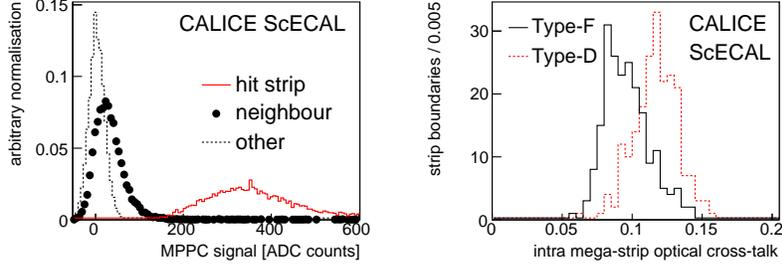
Figure 11: **Left:** Example of MPPC signal when a positron traversed a strip, a neighbouring strip within the same mega-strip or a non-neighbouring (other) strip. **Right:** Distribution of measured optical cross-talk between neighbouring strips in the same mega-strip.
