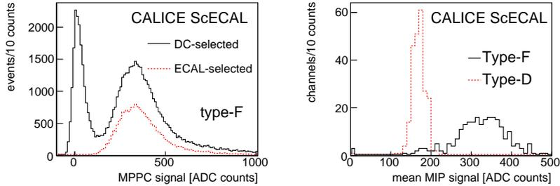
Figure 8: **Left:** ADC distribution for MIP runs, after drift chamber (DC) and ECAL based selections, for a representative type-F strip. **Right:** Distributions of the measured calibration constants for the two strip types.
