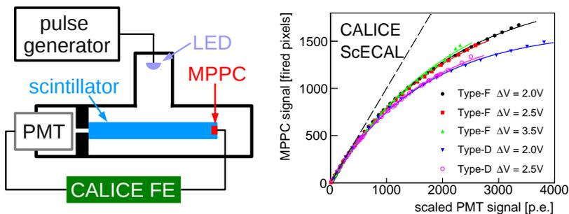
Figure 5: **Left:** The MPPC response curve measurement setup. **Right:** Measured MPPC response curves when using the two types of scintillator strips at different MPPC over-voltages  $\Delta V$ . The dashed line shows a linear response. Typical effective pixel numbers for the two types are given in Table 1.
