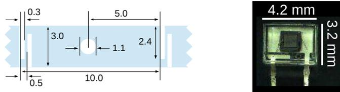
Figure 2: **Left:** Cross-section of one strip of the type-F mega-strip structure (all dimensions are in mm). The design of type-D mega-strips is the same, except without the hole. **Right:** Photograph of a MPPC. The package size is  $4.2 \times 3.2 \times 1.3 \text{ mm}^3$ , and the 1600 pixels are contained in an active area of  $1 \times 1 \text{ mm}^2$ .
