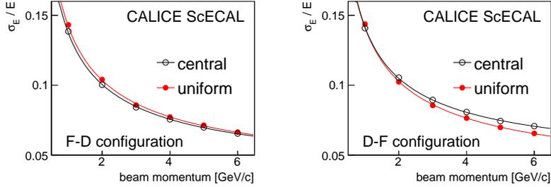
Figure 15: The energy resolutions measured using data taken with 1–6 GeV/c  $e^+$  beams in the central and uniform regions of the two detector configurations. The results of the fits described in the text are shown, and the fitted parameters reported in Table 2.
