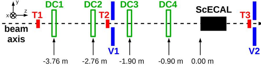
Figure 6: Sketch of the beam line instrumentation, showing the layout of the four pairs of drift chambers (DC1-4), three trigger counters (T1-3) and the two veto counters (V1-2) relative to the ScECAL prototype. (Not to scale.)
