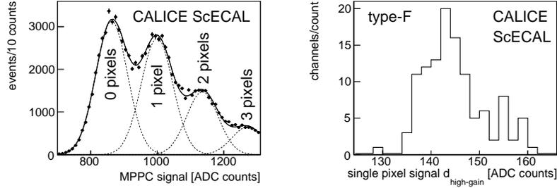
Figure 3: **Left:** A typical MPPC output spectrum taken with the LED system, showing the 0-, 1-, 2- and 3-fired-pixel peaks and the results of the fit. **Right:** Distribution of the measured single pixel signals  $d_{\text{high-gain}}$  in the type-F module with an MPPC over-voltage of 2.9 V.
