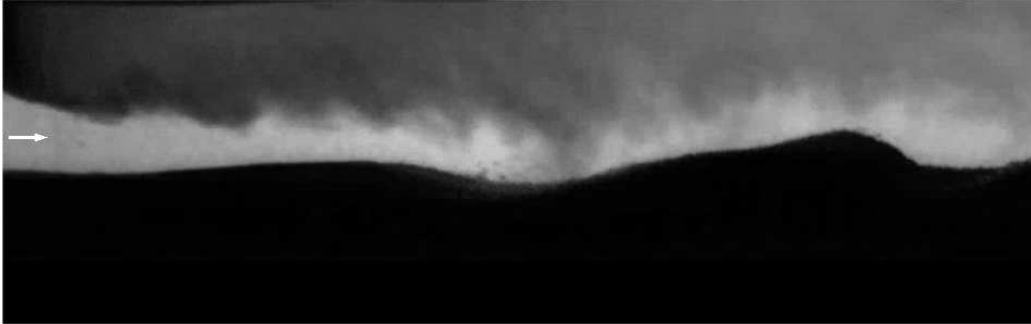
Figure 8: Snapshot of the fluid flow, when the upper layer was colored with ink. It can be seen that at the position of the second hole (at the center of the image) there is a strong mixing between the two layers, due to the turbulence that arise from the destabilization of the jet. It also visible that part of the sediment is lifted due to turbulent bursts.
