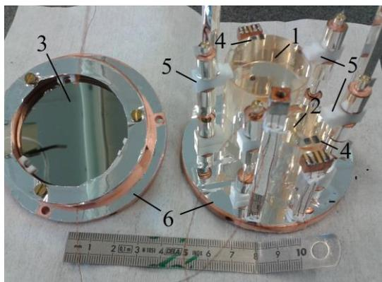
**Figure 4.** Photograph of the detectors setup: (1)  $\text{ZnMoO}_4$  crystal  $\text{Ø}35 \times 40$  mm; (2)  $\text{ZnMoO}_4$  crystal  $\text{Ø}20 \times 40$  mm; (3) Ge slab (photodetector); (4) NTD thermistors; (5) PTFE supporting elements; (6) Copper support of the detector covered by light reflector foil.
