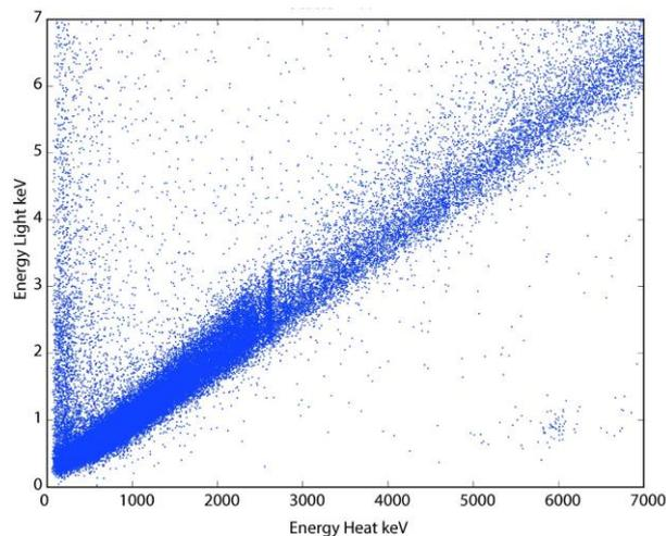
**Figure 6.** The scatter plot of light and heat signals for 160 g  $\text{ZnMoO}_4$  crystal accumulated over 81 h in aboveground set-up in Orsay. The  $\alpha$  band (populated mainly by  $^{210}\text{Po}$  internal contamination of the crystal) is neatly separated from the  $\beta$  band (containing also  $\gamma$  quanta and cosmic muons).
