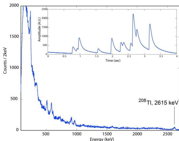
**Figure 5.** Energy spectrum accumulated by 160 g  $\text{ZnMoO}_4$  bolometer with  $^{232}\text{Th}$   $\gamma$  source. (Inset) Typical pile-up effect due to a slow time response of the bolometric detector.
