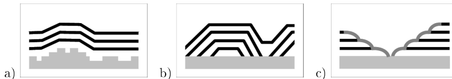
Figure 18: Expected result of graphene growth dominated by each of the three roughening mechanisms discussed in the text. (a) Germanium ejection might lead to graphene covering a roughened Ge substrate. (b) Chemical interaction between graphene edge and substrate dimers might lead to formation of multilayer graphene islands with bonded edges. (c) Migration of ejected Ge to graphene edges might lead to formation of Ge-rich facets terminating the multi-layer graphene islands.
