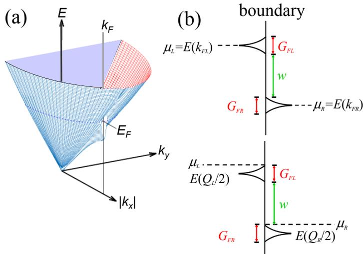
Fig. 1 (color online). (a) Schematic illustration of the Friedel gap at  $E_F$  for wave vectors perpendicular to an interface, assuming a linear unperturbed dispersion (e.g. that of graphene). (b) Schematics showing the Friedel gap shifting on two sides of an interface. Upper panel: Friedel gaps open at the respective chemical potentials, without considering the nonequilibrium effect of Friedel gap shifting. Lower panel: both gaps completely exist below their respective chemical potentials.
