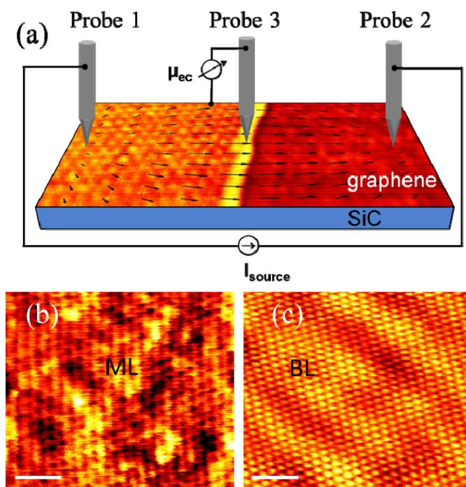
Fig. 2 (color online). (a) Schematic of the STP measurement setup. (b) STM images of ML and (c), BL graphene. Scale bar: 1 nm.
