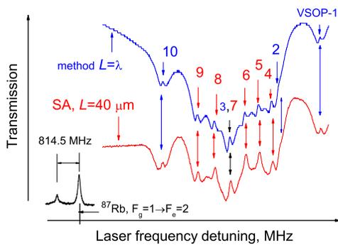
Fig. 4. Comparison of spectra for  $B = 5.6$  kG obtained with the NTC with the thickness  $L = \lambda$  (upper graph) and SA spectroscopy (middle graph) in the MTC with  $L = 40 \mu\text{m}$ . Laser power is  $1$  mW. The lowest curve is the reference.
