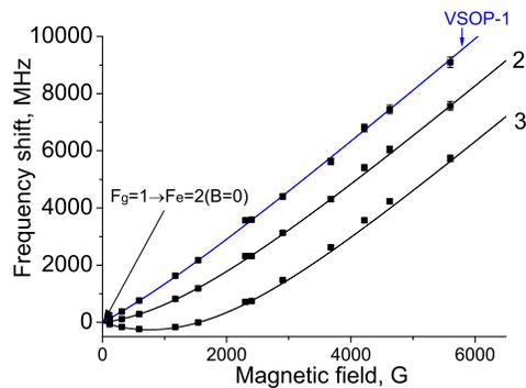
Fig. 5. Frequency shifts of the resonances labeled 1–3 [see Fig. 1(b)] in the magnetic field. Solid lines represent the theory and symbols correspond to the experimental results.
