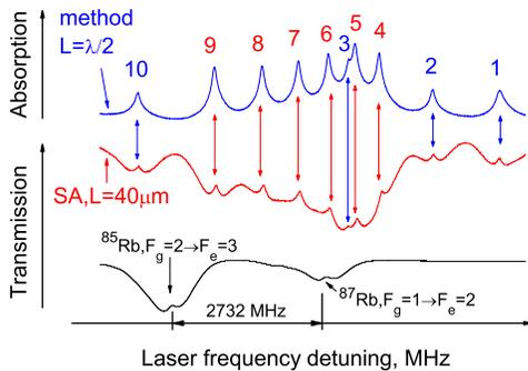
Fig. 3. Comparison of spectra for  $B = 2.2$  kG obtained with the NTC with the thickness  $L = \lambda/2$  (upper, blue curve; laser power  $50 \mu\text{W}$ ) and SA spectroscopy (middle, red curve) in the MTC (laser power  $1$  mW). The lowest curve is the reference.
