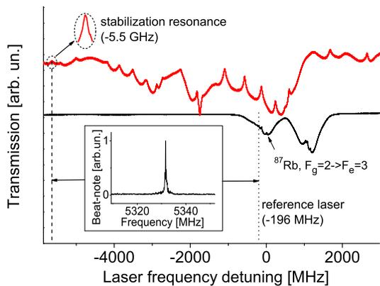
Fig. 6. SA spectrum of the rubidium  $D_2$  line in the MTC in  $B = 2.2$  kG (upper, red curve). Bottom (black) trace is the reference cell spectroscopy in  $B = 0$ . The resonance indicated by the dashed line was used for frequency stabilization of the diode laser. The inset graph shows the beat-note signal against a second, frequency locked (dotted line), laser.
