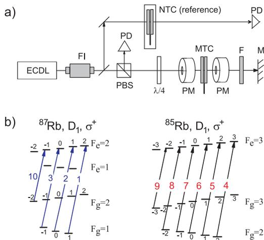
Fig. 1. (a) Sketch of the experimental setup. ECDL is the diode laser, FI - Faraday isolator, PM - permanent magnet,  $\lambda/4$  - quarter waveplate, PBS - polarization beam splitter, PD - photodetectors, F - filter, M - mirror; (b) Energy level diagram of the  $D_1$  line of the  $^{87}\text{Rb}$  (left) and  $^{85}\text{Rb}$  (right) in a magnetic field with the  $\sigma^+$  transitions of non-vanishing probability in the BG regime.
