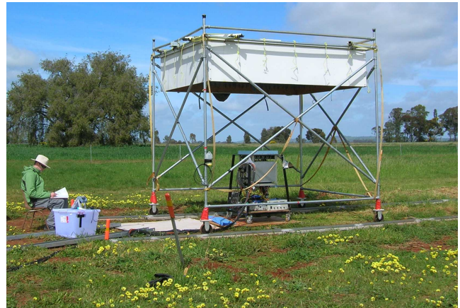
Figure 1. Absorber rolled over array under test at Parkes.
