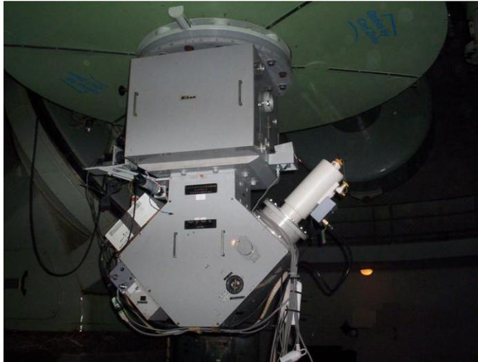
Fig. 5: OKS Spectrograph attached to the KAO's telescope
