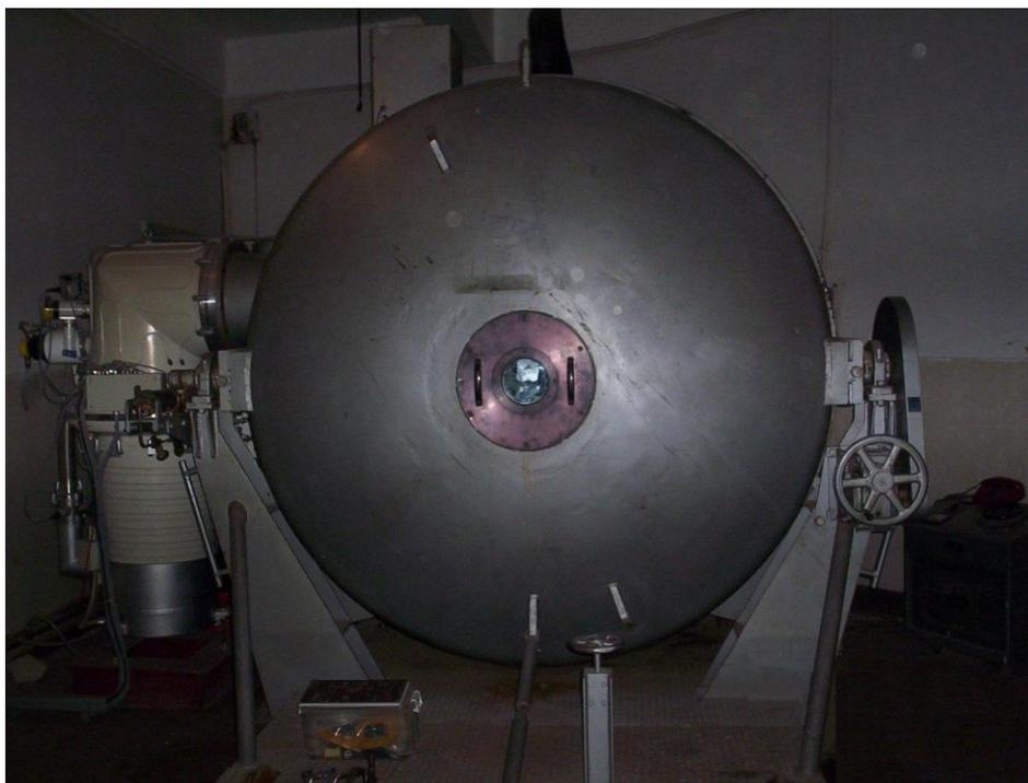
**Fig. 4: Upgraded Kottamia 74" mirror aluminizing plant**
