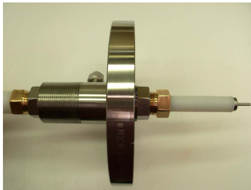
Figure 38: The NEXT-DEMO high-voltage feed-through, designed and built by Texas A&M
