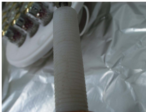
Figure 40: Detail of the carbon tracks produced in the polyethylene of the cathode feed-through during the tests in NEXT-DEMO.
