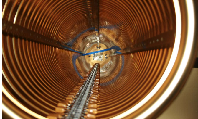
Figure 14: View inside the ARGONTUBE TPC at LHEP Bern. The Cockcroft-Walton, or Greinacher, circuit is supplying the high voltage to the field shaping rings.
