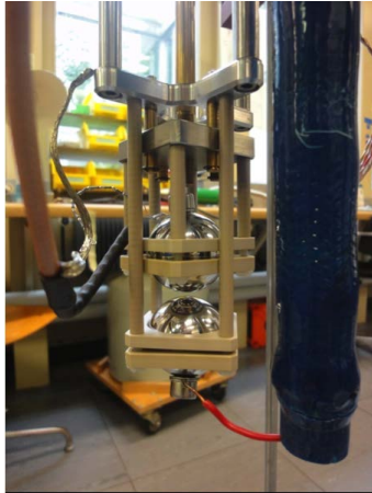
Figure 16: Breakdown measurements in liquid argon at the LHEP Bern using a maximum electric field of 30 kV and a maximum distance of 1 cm distance measured with micrometric precision.
