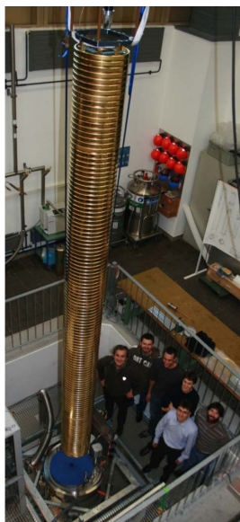
Figure 13: TPC of the ARGONTUBE at LHEP Bern. Gold plated field shaping rings to reduce high voltage breakdowns cover 5 m drift length.
