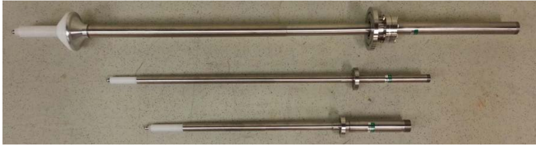
Figure 19: High voltage feed-throughs designed for the LBNE, DarkSide, and CAPTAIN liquid argon TPCs, from top to bottom.
