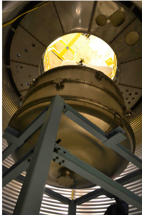
Fig. 4. The MiniCLEAN Outer Vessel on top of the detector stand inside the water shield tank in the SNOLAB Cube Hall.
