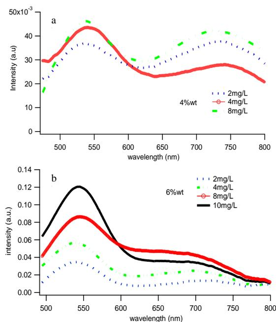
**Figure 5.** Optical extinction spectra of the nanocomposite films depending on the gold precursor concentration for a) 4%wt copolymer solution concentration and b) 6%wt copolymer solution concentration. On the graph b), one should notice that the 2mg/L and
