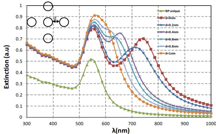
**Figure 6.** Optical extinction spectra of 10nm Au spheres calculated via the Discrete Dipole Approximation (DDA) model [9]. The optical extinction spectra are calculated for five nanoparticles displayed in staggered row and compared to the one of single nanoparticle. The surrounding medium is polystyrene and the distance  $d$  between the edges of two particles varies from  $d=0$ nm to  $d=1$ nm.
