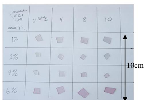
**Figure 2.** Aspect of the nanocomposite films composed of Au NPs organized into PS domains depending on both the concentration of polymers in the PGMEA solution and the density of added gold precursors. Thiolated PS was added to achieve a PS composition ratio of 20%.
