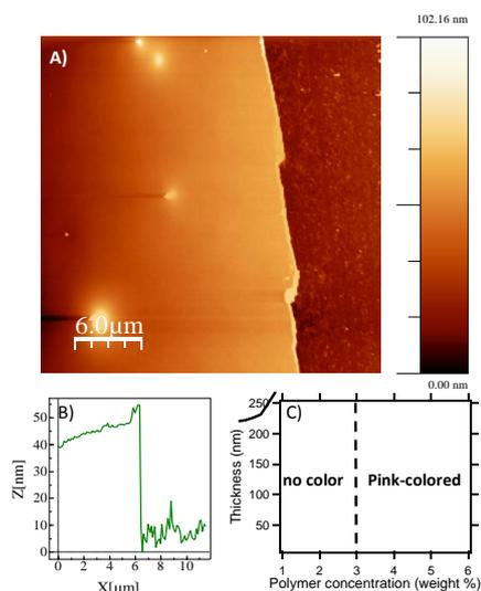
**Figure 3.** A) AFM image for polymer film thickness determination (3 % wt). B) Topography profile of a copolymer thin film obtained after spin-coating a 3 %wt polymeric solution. C) Thickness of polymer films as a function of %wt polymer solution. The polymer thin films become pink for 3 %wt or more polymer concentrations.
