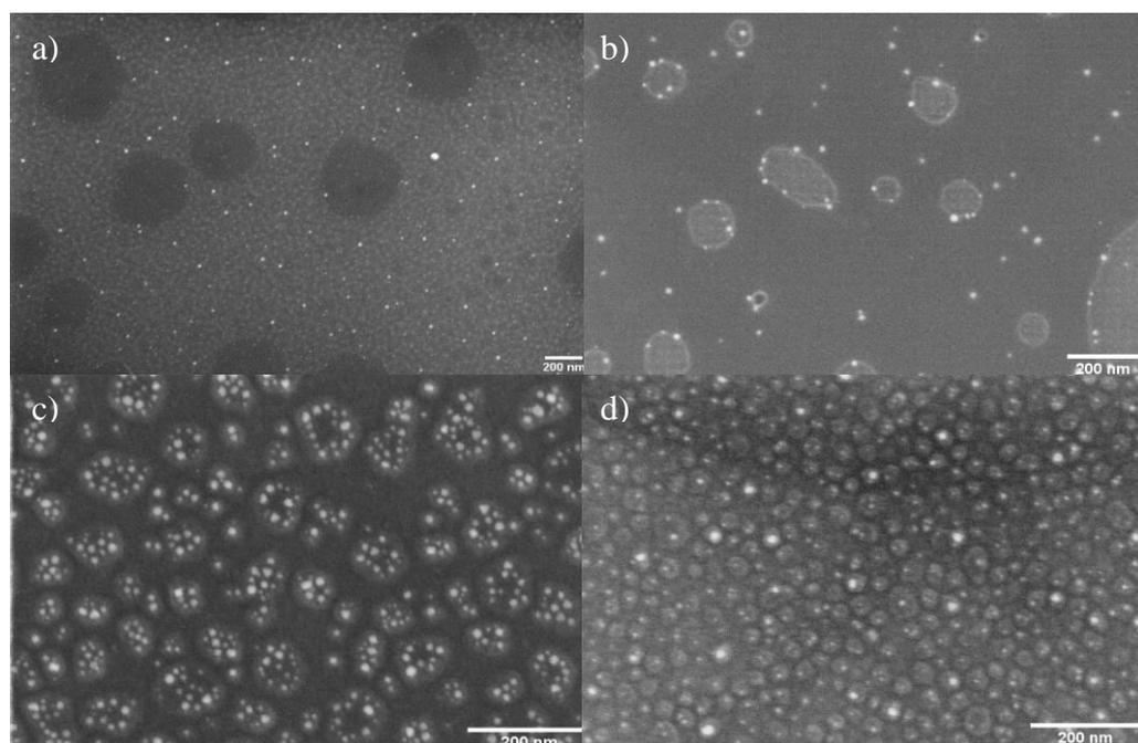
**Figure 1.** SEM images of Gold nanoparticles synthesized after microphase separation of copolymer thin films. The scale bars are 200nm large. a) no thiolated PS was added and PS domains were formed, b) no thiolated PS was added and PMMA domains were formed.
