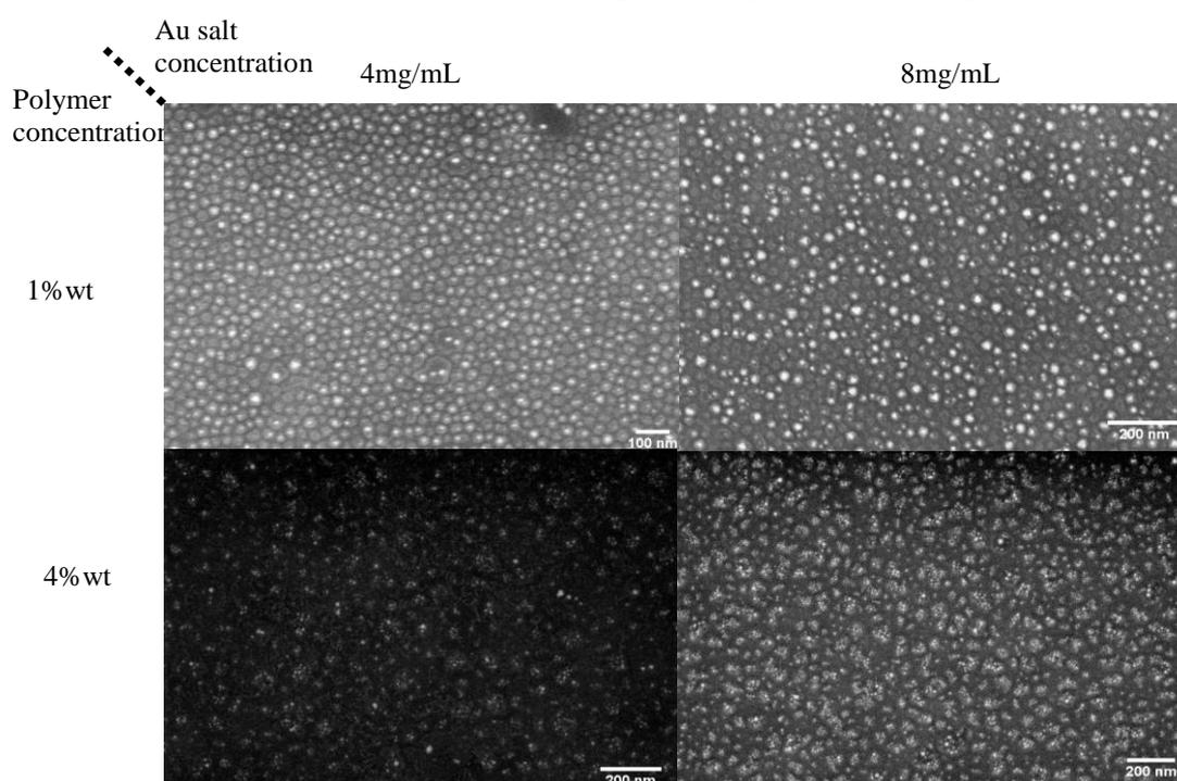
**Figure 4.** SEM images of the gold nanoparticles organized into the PS domains of the PS-PMMA block copolymer after microphase-separation (annealing at 200°C during 11 hours). The study of these images among others showed that increasing the solution concentration allows getting several Au NPs into the PS domains and that increasing the gold precursors concentration does not play any role in the Au NPs size.
