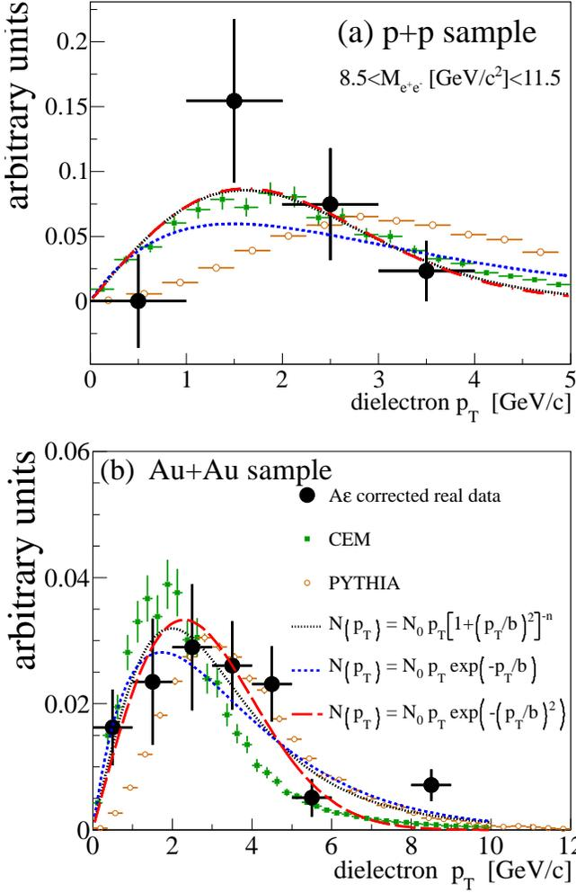
FIG. 8: (Color online) Transverse momentum dependence of acceptance corrected dielectron net counts in the  $\Upsilon$  mass region from  $p+p$  (a) and centrality integrated Au+Au (b) collisions. The lines are functions and  $\Upsilon$  yield estimations (Color Evaporation Model-CEM [62] and PYTHIA [61]) fitted to the distributions.
