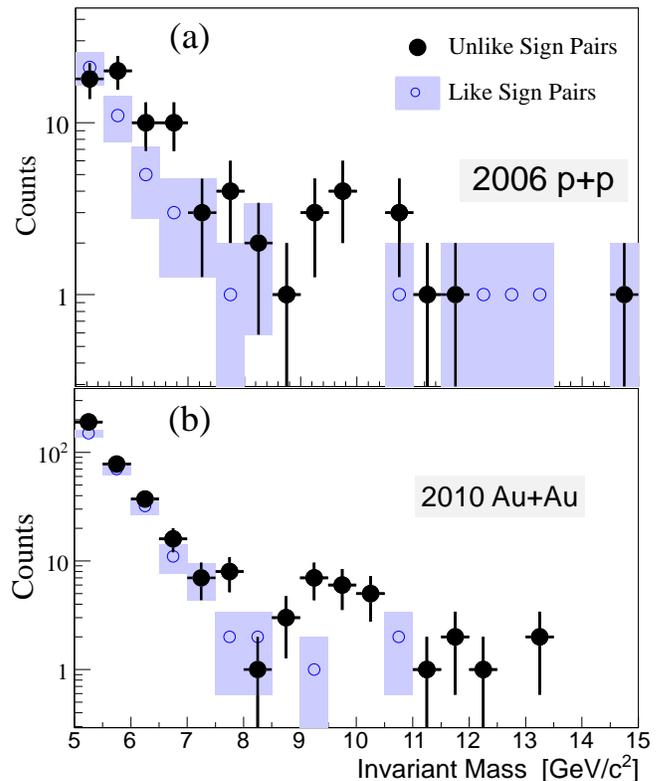
FIG. 5: Invariant mass distribution of unlike-sign and like-sign dielectrons in the  $\Upsilon$  mass region taken from  $p+p$  (a), and Au+Au collisions (b).
