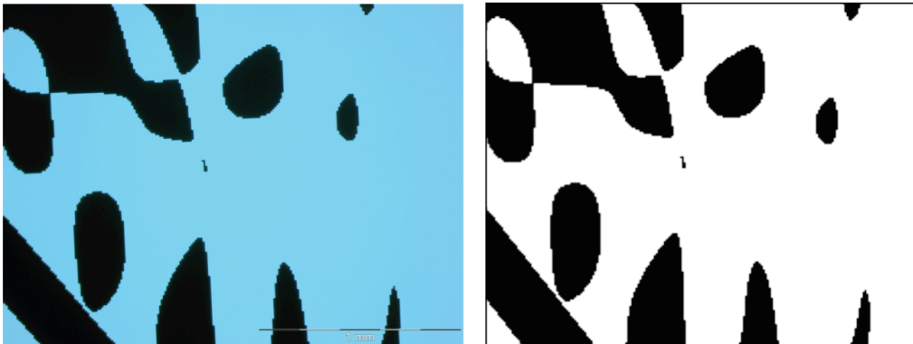
Figure 12: Comparison of the theoretical and actual transmissions of a portion of a 2D shaped pupil manufactured for the Subaru telescope. Left: microscope photography of the mask. Right: corresponding desired profile. Each pixel has a 10\mu m size.
