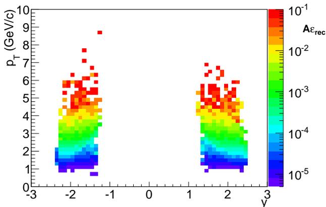
FIG. 5: (color online) The  $A\varepsilon_{\text{rec}}$  as a function of rapidity ( $x$ -axis) and  $p_T$  ( $y$ -axis) for  $\omega$ .
