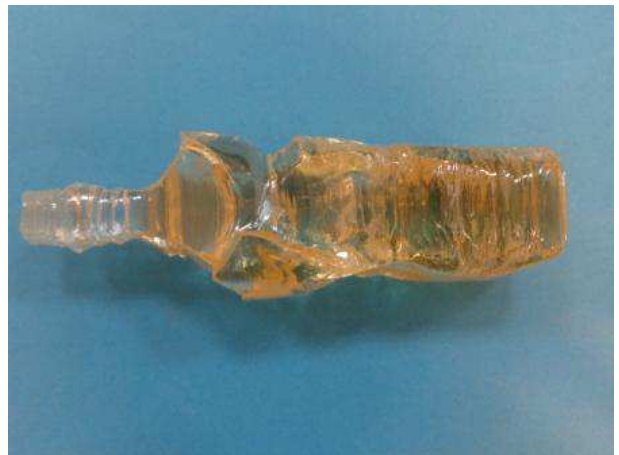
Fig. 1 Boule of \text{Zn}^{100}\text{MoO}_4 single crystal with mass of 170.7 g and length of 95 mm grown by the low-thermal-gradient Czochralski process.
