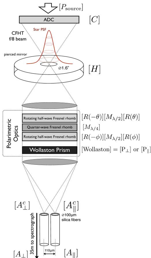
**Fig. 1.** Optical path of the polarimetric unit of ESPaDOnS.
