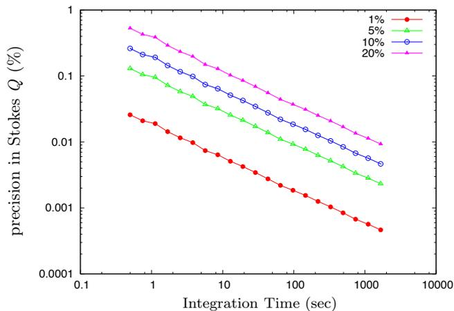
**Fig. 2.** Simulations of polarimetric precision in degree of polarization for Stokes  $Q$  versus integration time. These simulations only consider the effects caused by variability in fiber transmission. These results were obtained from 500 iterations, where we used four different values for the uncertainty in fiber transmission ( $\delta T$ ), 1%, 5%, 10%, and 20%, as indicated in the legend.
