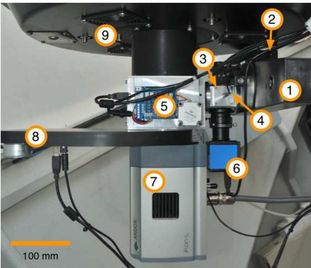
**Figure 4.** Imaging train: BACHES spectrograph (1), SBIG CCD camera (2), BACHES head (3), calibration fibre (4), GAM (5), slit view/guide camera (6), photometric CCD camera (7), filter wheel (8), telescope back plate (9).
