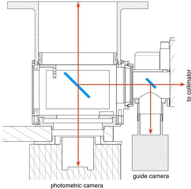
**Figure 6.** GAM ports configuration. Blue rectangles indicate mirrors.
