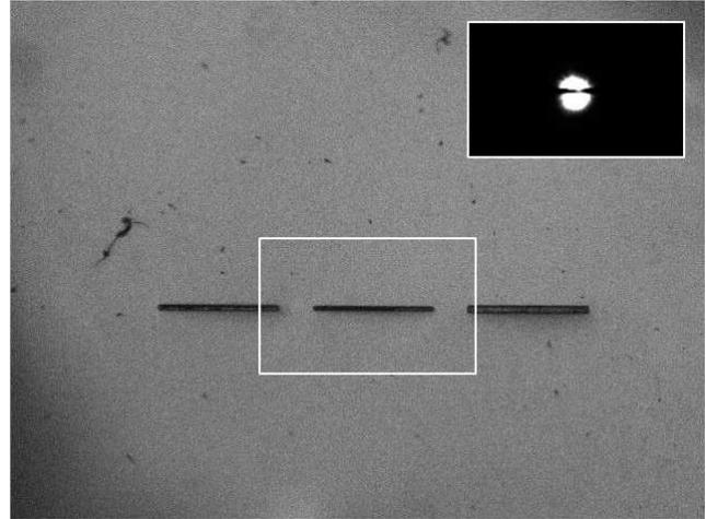
**Figure 7.** DMK guide camera image showing three slits – from left: 75, 25 and 100  $\mu\text{m}$ . Inset is a to-scale image of the star centred on the 25  $\mu\text{m}$  slit. Due to low, 8-bit depth of the image and the high contrast, the star appears overexposed.
