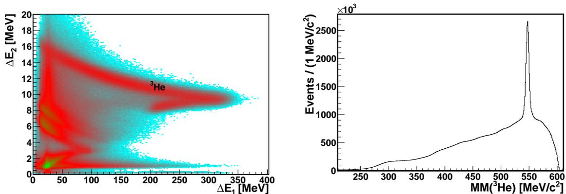
FIG. 1. (left) Correlation of energy deposits between two Forward Detector plastic detector layers: the first thick layer (11 cm),  $\Delta E_1$ , and a preceding thin (0.5 cm) layer,  $\Delta E_2$ . (right)  $MM({}^3\text{He})$  for all events with a  ${}^3\text{He}$  detected in the FD. There are about  $1.2 \cdot 10^7$  events in the peak corresponding to the  $pd \rightarrow {}^3\text{He}\eta$  reaction.
