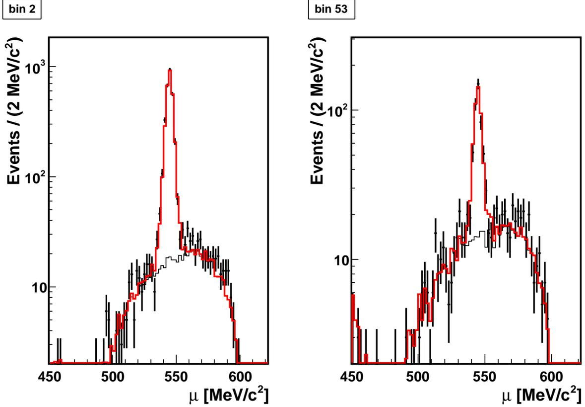
FIG. 5. Two examples of the fits to the  $dN/d\mu$  distributions for a large (left) and a low statistics Dalitz plot bin (right). The red thick line is the fitted function Eq. 7 while the thin line represents the continuous background contribution.
