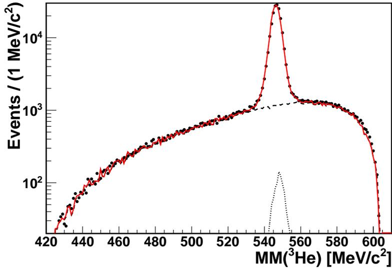
FIG. 3. The distribution of  $MM(^3\text{He})$  using variables adjusted by the kinematic fit for the final data sample (dots), agree well with the sum of the Monte Carlo distributions for the signal and the backgrounds (red solid line). Separately are shown contributions from  $\eta \rightarrow \pi^+\pi^-\gamma$  (dotted line) and from the direct  $3\pi$  production (dashed line).
