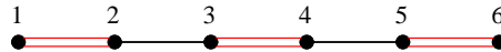
Figure 2. Effective dimerized chain corresponding to the ribbon shown in Figure 1. Single black lines: unit hopping amplitudes. Double red lines: \gamma hopping amplitudes.
