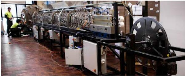
Figure 7. Device for assembling 15/5 (15 strands with 5 mm width) Roebel cables (courtesy IRL-General Cable).
