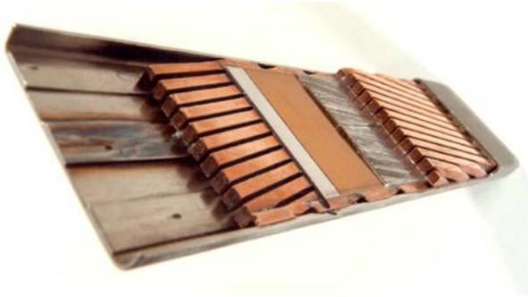
**Figure 2.** The NbTi Roebel cable of the EURATOM toroidal field magnet in the Large Coil Task project [9].
