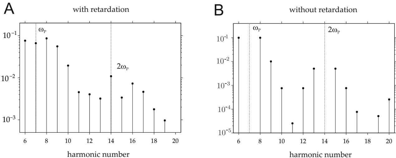
FIG. 3. **Harmonic spectra from the ROM model using two oscillations at  $\omega_L$  and  $\omega_P$ :** The parameters are taken from the PIC simulation ( $\omega_P = 7\omega_L$ ,  $a_L = 0.1c/\omega_L$ ,  $a_P = 0.1c/\omega_P$ ,  $\varphi_L = 0$ ,  $\varphi_P = 0$ ).
