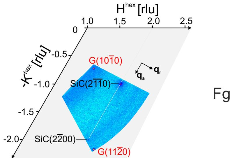
FIG. 3. Reciprocal space map of monolayer graphene/BL on SiC(0001). The axes are scaled with the reciprocal lattice units (rlu) of SiC,  $q_a$  and  $q_r$  mark the radial and angular directions in the RSM.
