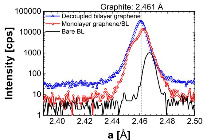
FIG. 4. Line scans through the  $G(11\bar{2}0)$  reflection along  $q_r$ , transformed to real-space, performed for the bare BL, monolayer graphene/BL, and bilayer graphene samples. The dotted line indicates the value for the lattice parameter of graphite.<sup>31</sup> The x-axis is scaled to the lattice parameter of graphene.
