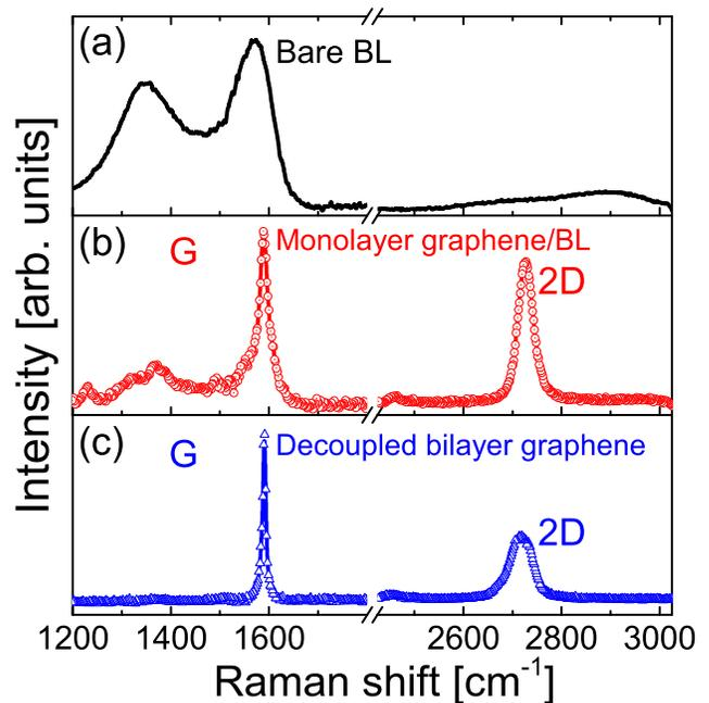
FIG. 2. Raman spectra of the three samples investigated in the present study: (a) bare BL; (b) monolayer graphene on top of the BL; (c) bilayer graphene on top of an oxidized SiC surface (obtained by oxygen intercalation upon air annealing).
