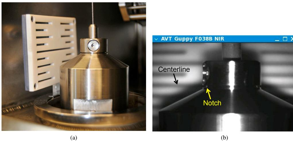
Figure 7: Two images of the weight in its “tare” position, in which the notch in the weight’s neck is aligned with the long centerline in the camera backdrop. (a) Photo of the weight and ruled backdrop inside the MiniCal housing. (b) The same scene as viewed through the camera. The backdrop’s hash marks are spaced at 5 mm intervals.
