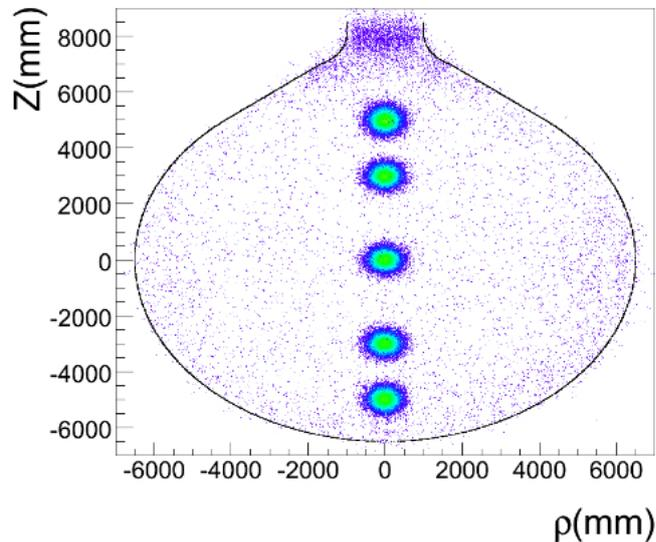
Figure 8: Activity from a  $^{60}\text{Co}$  source deployed to  $z = +5, +3, 0, -3, -5$  m along the detector's  $z$ -axis, as reconstructed from the data. The colors correspond to the intensity of detected activity.
