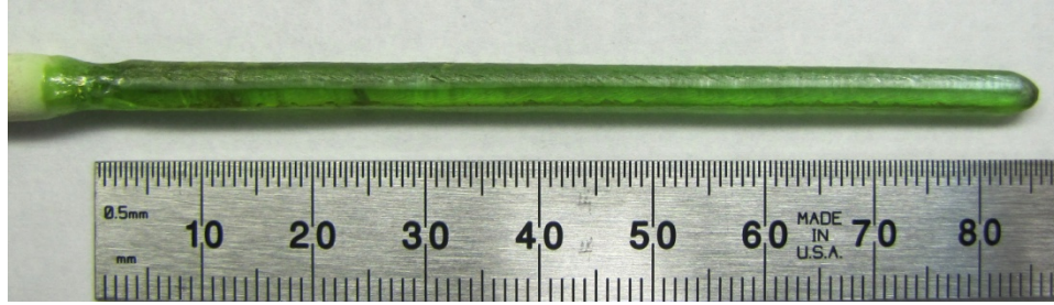
Fig. 4. A typical Pr 2 Zr 2 O 7 single crystal grown under 1 bar static high-purity argon atmosphere using an optical floating zone image furnace.
