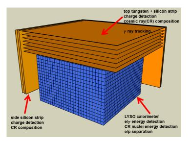
Figure 1. Schematic diagram of HERD.
