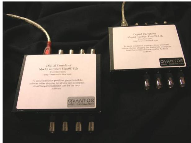
Figure 1. Digital photon correlators of the type used in present laboratory experiments. These are based upon Field Programmable Gate Arrays (FPGA) with 700 MHz clock rate, 1.4 ns time resolution, handling up to 200 MHz photon-count rates at TTL-level voltages. Each of these correlators handles signals from eight telescopes simultaneously.
