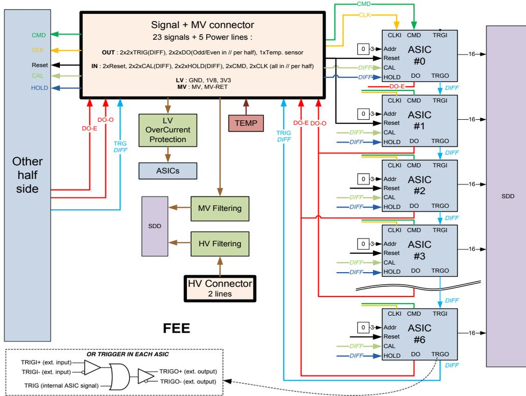
Figure 2. Schematic drawing of the interface between the FEE and (M)BEE showing the signals to and from the ASICs.
