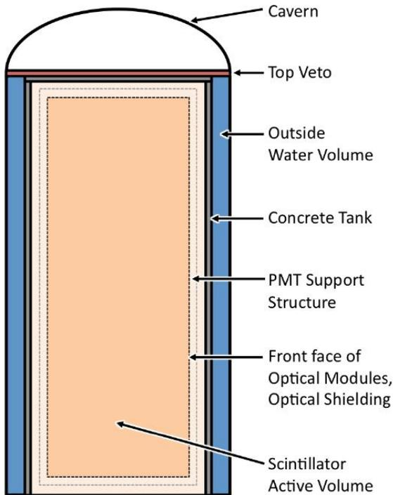
FIG. 1. Schematic view of the LENA detector [5].
