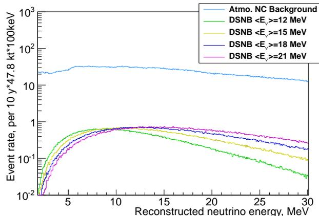
FIG. 4. The simulated atmospheric neutrino NC background spectrum. For comparison, the DSNB spectra with  $\langle E_\nu \rangle$  ranging from 12 MeV to 21 MeV are also depicted.
