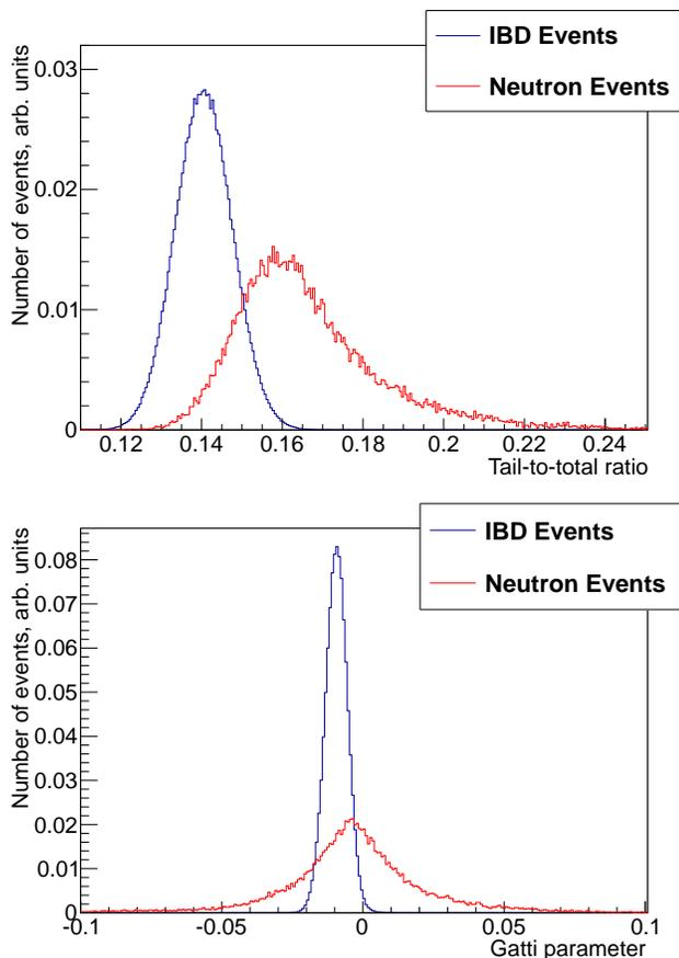
FIG. 7. The tail-to-total ratio (upper plot) and gatti parameter (lower plot) distribution for IBD (denoted in blue) and neutron events (denoted in red) in the center of LENA with  $E_{\text{vis}} = 9.2$  MeV.
