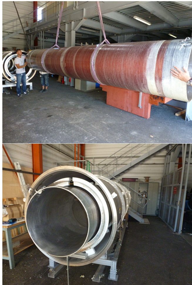
Figure 2. Upper picture: The 5 m long copper-wired solenoid. Lower picture: the solenoid inserted into the 4 meter long \mu -metal magnetic shield.
