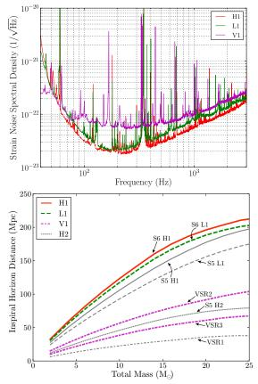
**Figure 1.** Typical detector strain noise spectral density for the LIGO S6 and Virgo VSR2+3 runs, as well as the best equal-mass binary coalescence horizon distance achieved for each run as a function of total system mass. The horizon distance is the distance at which an optimally oriented binary merger would produce an expected signal-to-noise of 8. Figures reproduced from (Abadie *et al.* 2012)
