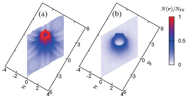
FIG. 4: (Color online) Local ZDOS landscapes around a vortex core for the band-1 (a) and band-2 (b) with  $\mu = 1$  at  $\bar{B} = 0.15$  and  $T = 0.2T_c$ . One unit cell of the triangular vortex lattice is shown with the length measured by  $\xi_0$ .
