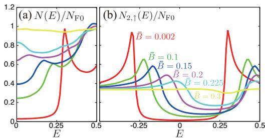
FIG. 3: (Color online) Total DOS  $N(E)$  (a) and DOS for up spin component in band-2  $N_{2,\uparrow}(E)$  (b) for various  $\bar{B}$  with  $\alpha_M = 1.76$  at  $T = 0.2T_c$ . At  $\bar{B} = 0.002$ ,  $\Delta_1 = 0.58$  and  $\Delta_2 = 0.29$ . By increasing  $\bar{B}$ , the gap edge singularities corresponding to the minor gap  $\Delta_2$  move inward to  $E = 0$ . At  $\bar{B} = 0.225$ , total DOS has a maximum at  $E = 0$ .
