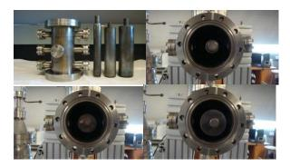
FIG. 3. Cylindrical cavity and inner electrodes with varying diameter. In clockwise direction: the disassembled arrangement and three end on views of the assembled electrode configuration, starting with the lowest diameter of the electrode.
