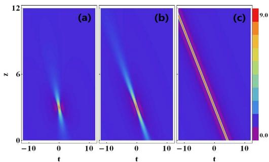
FIG. 2: Transition of first-order localized waves  $|E_1(t, z)|^2$  from rogue wave to w-shaped traveling wave: (a)  $q = 0$ , (b)  $q = q_s/2$ , (c)  $q = q_s$ , all obtained under  $a = 1$ ,  $\beta = 0.1$ ,  $z_0 = 3$ , and  $t_0 = 0$ . This corresponds to the process from MI region to stability line described by the arrows in Figure 1(b). Here (a) and (b) show the classical tilted rogue waves in the HE, while (c) shows a w-shaped traveling wave.
