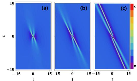
FIG. 6: Transition of second-order waves  $|E(t, z)|$  with (a)  $q = 0$ , (b)  $q = q_s/2$ , (c)  $q = q_s$ , all obtained under  $a = 1$ ,  $\beta = 0.1$ ,  $z_0 = 0$ , and  $t_0 = 0$ . (a) and (b) show the second-order rogue waves with a single peak, and the maximum peak value is always 5 times of the background. (c) shows the local structure of localized wave interaction in stability region.
