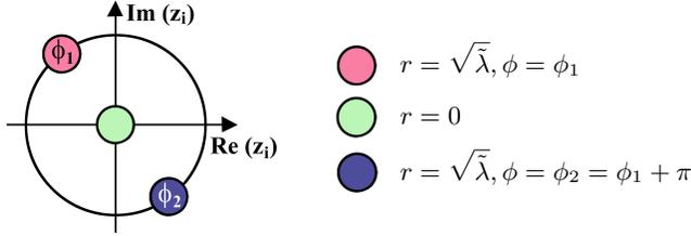
FIG. 2. (color online) Sketch of the different oscillator groups occurring in an eigensolution. The red (dark grey) and blue (black) group are on the limit cycle given by Eq. (13) with phase difference  $|\phi_1 - \phi_2| = \pi$ . Oscillators of the green (light gray) group are in the steady state at  $z_i = 0$ .
