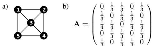
FIG. 1. **a)** Motif of 5 coupled oscillators given by the normalized adjacency matrix,  $A$ , shown in **b)**. It is used in this paper for illustrating general results that can be applied to all undirected motifs.
