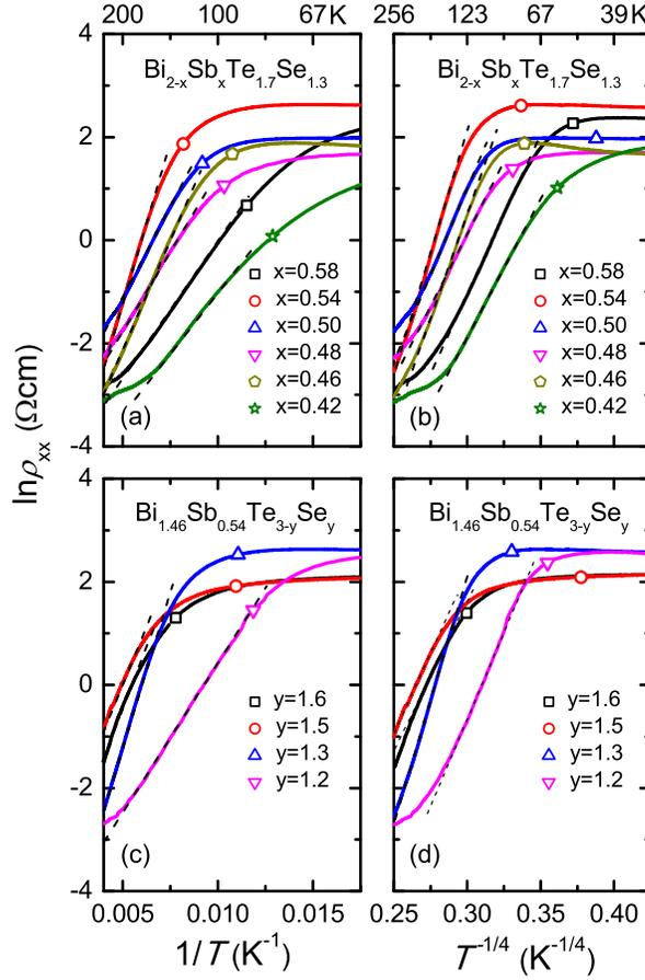
**Figure 2.** Temperature variation of the resistivity of BSTS in a plot of  $\ln \rho_{xx}$  versus  $1/T$  in frames (a) and (c), and versus  $T^{-1/4}$  in frames (b) and (d). The linear dashed lines represent the activation behavior and the 3D VRH behavior (see text). In frames (a) and (b) we have traced the resistivity for  $y = 1.3$  and  $x$ -values as indicated, and in frames (c) and (d) the resistivity for  $x = 0.54$  and  $y$ -values as indicated.
