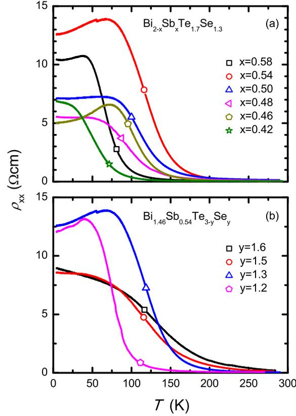
**Figure 1.** Temperature dependence of the resistivity of  $\text{Bi}_{2-x}\text{Sb}_x\text{Te}_{3-y}\text{Se}_y$  crystals with (a)  $y = 1.3$  and  $x$ -values as indicated, and (b)  $x = 0.54$  and  $y$ -values as indicated. The typical sample thickness is  $100 \mu\text{m}$ .
