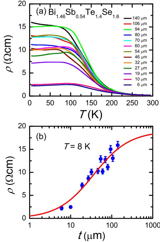
**Figure 4.** (a) Temperature dependence of the resistivity of a  $\text{Bi}_{1.46}\text{Sb}_{0.54}\text{Te}_{1.4}\text{Se}_{1.6}$  crystal with thickness  $t = 140 \mu\text{m}$  thinned down in 12 steps to  $6 \mu\text{m}$  as indicated. (b) Measured resistivity at 8 K as a function of thickness (solid dots). The solid line represent a fit of the data to the parallel resistor model (see text).
