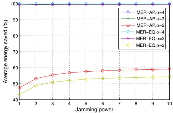
Fig. 7. Average energy saved vs. jamming power of each malicious jammer for different values of the path-loss exponent.  $n_j = 20$  number of jammers,  $n = 20$  system nodes, and end-to-end target probability of outage  $\pi = 0.1$  are considered. The system nodes and the jammers are placed uniformly at random over a  $10 \times 10$  square.
