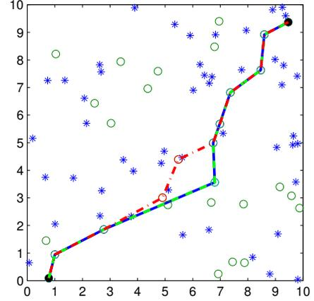
Fig. 5. A snapshot of the network with the same system node and jammer placement as in Fig. 4. Transmit power of each jammer  $P_j = 1$ , target outage probability  $\pi = 0.1$ , and transmission in a lossy environment is considered ( $\alpha = 4$ ). The MER-AP path is shown by the dashed line (green), the MER-EQ path is shown by the solid line (blue), and the MER path is shown by the dash-dotted line (red). The energy saved in this network for MER-AP is 93.54% and for MER-EQ is 88.21%.
