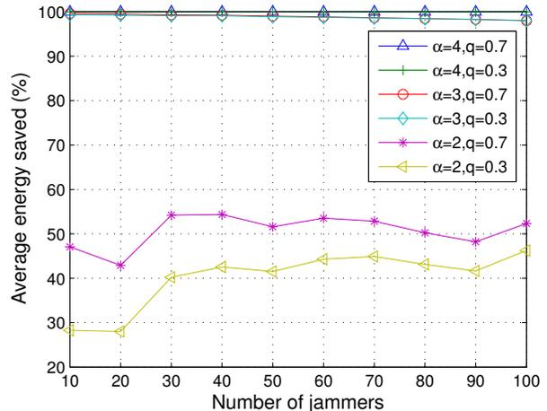
Fig. 13. Average energy saved vs. number of dynamic jammers for different values of the path-loss exponent and probability  $q$  of a jammer being in “ON” state. The transmit power of each jammer  $P_j = 1$ , the target end-to-end outage probability  $\pi = 0.1$ , and  $n = 20$  system nodes are considered. The system nodes and the jammers are placed uniformly at random over a  $10 \times 10$  square.
