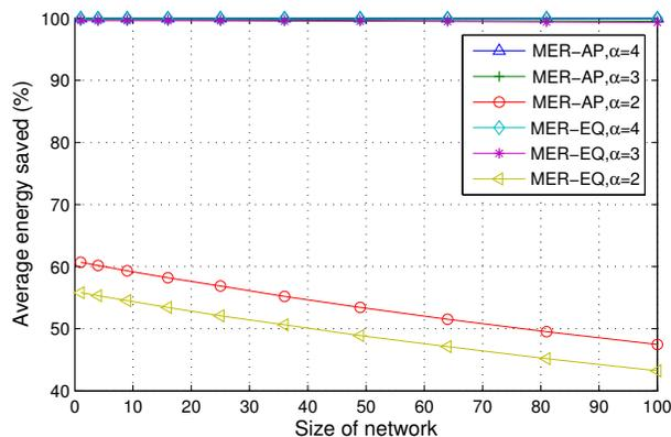
Fig. 8. Average energy saved vs. area of the network for different values of the path-loss exponent. The transmit power of each jammer  $P_j = 1$ ,  $n_j = 20$  number of jammers,  $n = 20$  system nodes, and end-to-end target probability of outage  $\pi = 0.1$  are considered.
