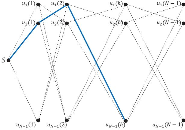
Fig. 1. Network expansion: add  $N - 1$  replicas for each node  $u_i$ ,  $i = 1, \dots, N - 1$  to the expanded network. Then links (shown by dashed lines) are added to the expanded network such that a path from  $S$  to  $u_i(h)$  will have exactly  $h$  hops. Hence, every path from  $S$  to  $D(h)$  has exactly  $h$  hops. A sample path from the source to  $u_{N-1}(h)$  is shown by bold solid lines.
