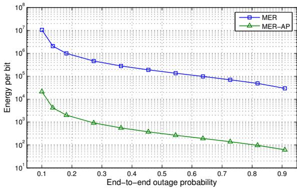
Fig. 12. Energy per bit versus the end-to-end outage probability for MER-AP and MER. The throughput is measured for five concurrent flows, where  $n = 10$  system nodes and  $n_j = 20$  jammers are present in the system. The amount of energy per bit MER-AP uses is about two orders of magnitude less than MER.
