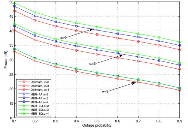
Fig. 3. Total power versus outage probability for brute-force 'exact' algorithm (optimum), MER-AP, and MER-EQ.
