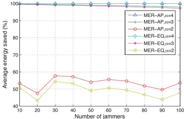
Fig. 6. Average energy saved vs. number of static jammers for different values of the path-loss exponent. The transmit power of each jammer  $P_j = 1$ , the end-to-end target probability of outage  $\pi = 0.1$ , and  $n = 20$  system nodes are considered. The system nodes and the jammers are placed uniformly at random over a  $10 \times 10$  square.
