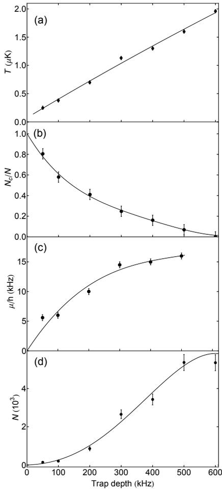
FIG. 7. Variation of (a) temperature  $T$  (b) condensate fraction  $N_c/N$  (c) chemical potential  $\mu/h$  and (d) atom number per site  $N$ , with trap depth for lattice site 38 with  $\omega_{rad}/2\pi = 7.5$  kHz,  $\omega_{ax}/2\pi = 260$  Hz. The points were determined from fits to the RF spectra in Fig. 6, as described in the text. The solid lines are polynomial fits constrained to pass through (b)  $N_c/N = 1.0$  (c)  $\mu/h = 0$  and (d)  $N = 0$  at zero trap depth.
