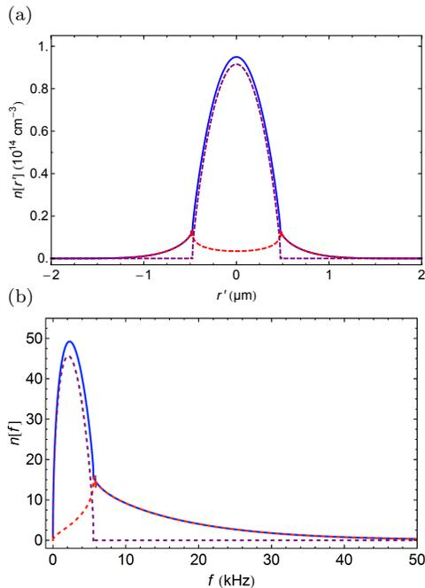
FIG. 2. (Colour online) Calculated (a) atom density versus  $r'$  and (b) RF spectrum, showing the contribution of the BEC alone (dashed purple line), the thermal cloud alone (dashed red line) and the sum of the two (blue solid line) for  $^{87}\text{Rb}$   $|F=1, m_F=-1\rangle$  atoms confined in a magnetic trap. Parameters:  $T = 0.5 \mu\text{K}$ ,  $\mu/h = 7.5 \text{ kHz}$ ,  $\bar{\omega}/2\pi = 2.40 \text{ kHz}$ ,  $a_s = 5.3 \text{ nm}$ .
