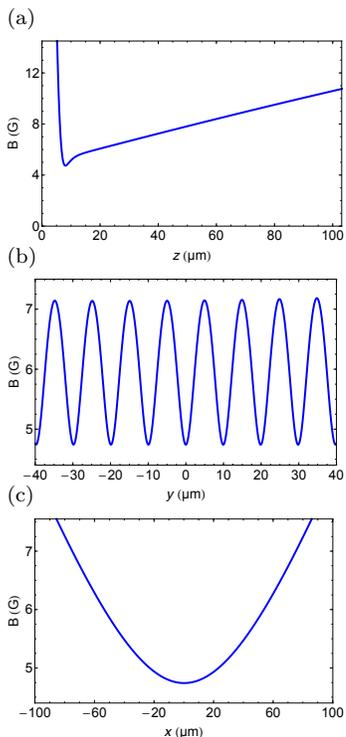
FIG. 3. Simulations of the magnitude of the magnetic field along the (a)  $z$  (b)  $y$  and (c)  $x$  directions of the lattice microtraps using the RADIA code [19]. Parameters:  $4\pi M_z = 3$  kG,  $t = 0.96$   $\mu\text{m}$ ,  $a = 10$   $\mu\text{m}$ ,  $I_z = 17$  A,  $B_{bx} = 51$  G,  $B_{by}^c = 0$ .
