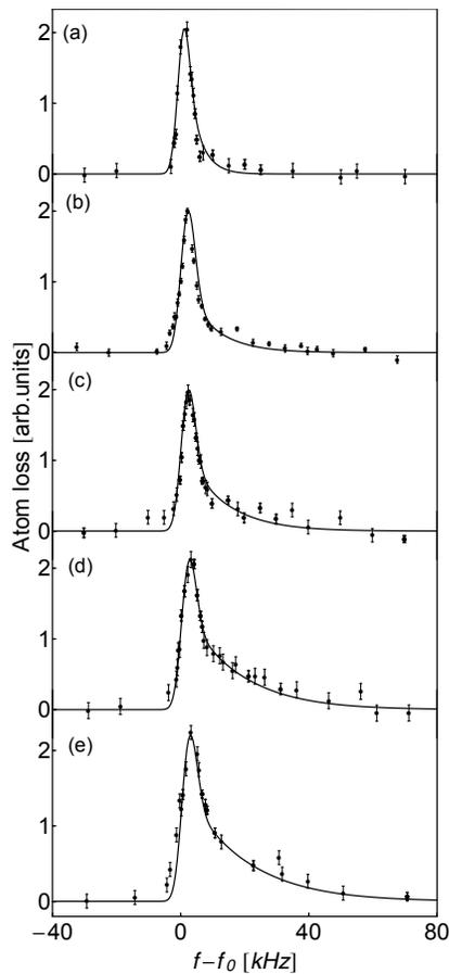
FIG. 9. RF spectra of loss of atoms in lattice site 38 for different radial trap frequencies of (a) 1.5 kHz (b) 7.5 kHz (c) 9.5 kHz (d) 16.1 kHz and (e) 19.9 kHz, with  $\omega_{ax}/2\pi = 260$  Hz,  $\delta f = 100$  kHz. The solid lines are fits to the data points based on the self-consistent mean-field model for a BEC plus thermal cloud convoluted with a Gaussian magnetic noise function with FWHM = 4.3 kHz, as described in the text.
