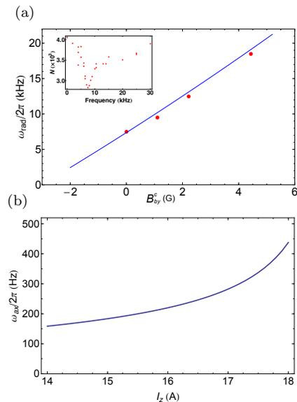
FIG. 4. (a) Radial trap frequency of the magnetic lattice traps versus  $B_{by}^c$  provided by external coils for  $I_z = 17$  A,  $B_{bx} = 51$  G measured by parametric heating. The solid line represents the calculated radial trap frequency over the range used in the experiments. The inset shows the parametric heating resonance for  $B_{by}^c = 0$ . (b) Calculated axial trap frequency versus  $I_z$  for  $B_{by}^c = 0$ ,  $B_{bx} = 51$  G.
