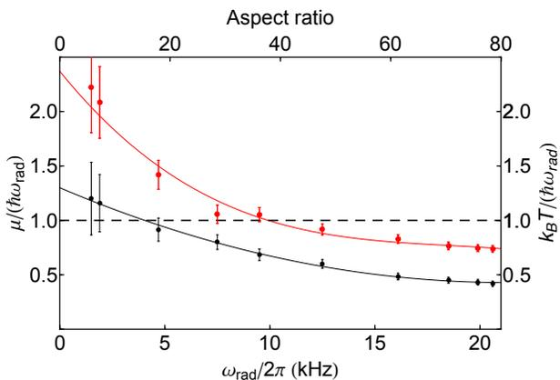
FIG. 11. (Colour online)  $\mu/(\hbar\omega_{rad})$  (black points) and  $k_B T/(\hbar\omega_{rad})$  (red points) versus radial trap frequency for  $\omega_{ax}/2\pi = 260$  Hz,  $\delta f = 100$  kHz. The region where both black and red points lie below the dashed line indicates the quasi-1D Bose gas regime. The solid lines are polynomial fits to the data points.
