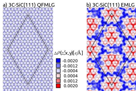
FIG. 4: Electron density differences  $\Delta\rho(r) = \rho_{\text{full}}(r) - (\rho_{\text{G}}(r) + \rho_{\text{sub}}(r))$  for (a) 3C-SiC QFMLG and (b) 3C-SiC EMLG, calculated in the  $x$ - $y$ -plane between the substrate and the graphene layer (1.08 Å below the graphene layer). The ( $6\sqrt{3} \times 6\sqrt{3}$ )-R30° supercell is shown in black and the graphene layer in gray.
