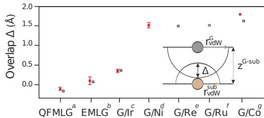
FIG. 3: Comparison of the overlap  $\Delta$  for different epitaxial graphene systems.  $\Delta$  is calculated by subtracting  $z^{G-sub}$  from the sum of graphene and substrate vdW radii. The empty and the filled squares correspond to DFT and measured values, respectively.  $a$ : this work,  $b$ : [31, 32],  $c$ : [5],  $d$ : [6],  $e$ : [33],  $f$ : [34],  $g$ : [35].
